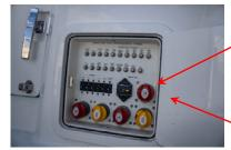
2 Ensure that the "House" battery switch is on at the main D.C. panel to feed power to all of the manual circuit breakers on the D.C. panel.
