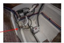
1 Ensure that the sewage tank discharge seacock is open.
