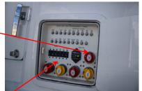
3 Ensure that the "Elect" (to feed the fuse block for the monitors and other electronics) 50a, "COI 1" (to feed COI1 D.C. Loads) 100 a, "COI 2" (to feed COI2 D.C. loads) 100 a, "OI" (LROI 20a), and "C6" (5a Output Interface) manual circuit breakers are on at the main D.C. panel. These circuit breakers feed the D.C. loads and NMEA 2000 bus of the Czone system.
