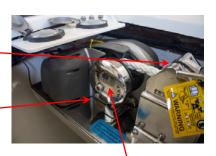
9 When safe insert the Lewmar wrench into the keyed hole in the face of the free fall cap and rotate clockwise to grip the gypsy and anticlockwise to free the gypsy
