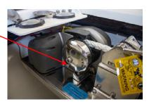
switch until the anchor is under free fall. If the clutch was left in a locked position the anchor will start to fall almost immediately. If unlocked it could take several seconds to fully re-engage the internal clutch. NOTE: Pressing the DOWN button for over 5 seconds will result in a longer clutch re-engagement time during the next UP command.
