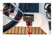
29 Pushing the Ignition button turns the power to each engine ON and OFF. When the power is ON, the active indicator will be illuminated. Turning the Ignition buttons on powers up the Helm Master system.
