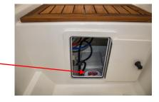
discharges out the stbd. hull side aft. The bilge level alarm switches are beside the aft pumps.
