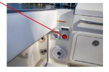
23 Once the cable is fully retracted close the cap on the transom entrance hole.
