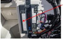
6 Ensure that the green network LEDs on the COIs are on indicating that the Czone NMEA network is intact.
