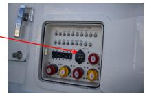
10 Set the Czone boat Mode of Operation to "All Off" as desired if leaving the boat. In the "All Off" mode the automatic bilge pump, high water alarm, and stereo memory circuits will remain energized unless their pop out type circuit breakers on the main D.C. panel are turned off.
