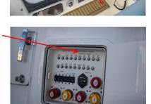
3 Ensure that the "House" battery switch is on at the main-D.C. panel to feed power to all of the manual circuit breakers on the D.C. panel except the "Continuous Power" circuit breakers which are fed direct from the house batteries all the time.
