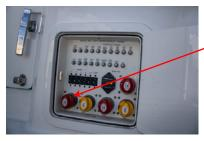
3 Ensure that the port start battery switch is on in the main D.C. panel
