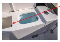
6 Rotate the knob on the port side of the inside of the chiller box clockwise
