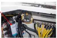
**LOCATION:** The raw water wash down pump is inboard under the port aft deck in the "Mechanical room". The raw water suction seacock is on the raw water seachest in the compartment with it. The raw water wash down connections are on the aft deck and in the port bow hatch.
