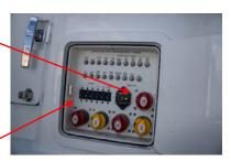
4 Ensure that the "Elect" (to feed the fuse block for the monitors and other electronics) 50a, "COI 1" (to feed COI1 D.C. Loads) 100 a, "COI 2" (to feed COI2 D.C. loads) 100 a, "OI" (LROI 20a), and "C6" (5a Output Interface) manual circuit breakers are on at the main D.C. panel. These circuit breakers feed the D.C. loads and NMEA 2000 bus of the Czone system.
