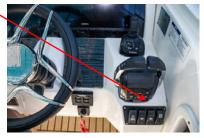
12 The joystick switch transfers boat operation from the remote control and steering
