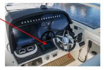
5 Trim assist mode does not operate in the free throttle mode and joystick mode. Only pushing the trim assist switch exits from trim assist mode. The active indicator will go out. When the trim assist function has been switched ON, it will remain active until cancelled by the operator even when turning the ignition switch OFF and back to ON.
