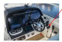
4 Operate the helm seat with the rocker switch to stbd. of the helm on the main control console.
