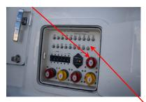
3 Ensure that the 12 volt "House" battery voltage is adequate (at least 12 volts).
