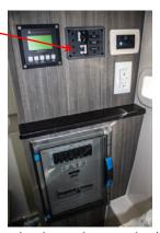
6 Ensure that the "Elect" (to feed the fuse block for the monitors and other electronics) 50a, "COI 1" (to feed COI1 D.C. Loads) 100 a, "COI 2" (to feed COI2 D.C. loads) 100 a, "OI" (LROI 20a), and "C6" (5a Output Interface) manual circuit breakers are on at the main D.C. panel. These circuit breakers feed the D.C. loads and NMEA 2000 bus of the Czone system.
