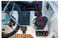
helm to the joystick. While the engine is running, placing the remote control lever and the joystick lever in the N position and pushing the joystick switch enters the joystick mode, allowing operation with the joystick lever. The active indicator illuminates during operation. While in the joystick mode, the engine speed is limited and the steering wheel is locked.
