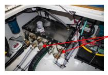
4 The air conditioning raw water pump supply
