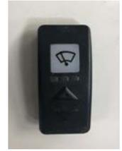
This switch will activate the rinse system included in the wiper option. The rinse system is tied into the freshwater supply on the vessel. In-order for the rinse system to function properly the fresh water pump must be turned on. The fresh water pump switch is a labeled push button mechanical switch located on the dash of the 280DC-X.
