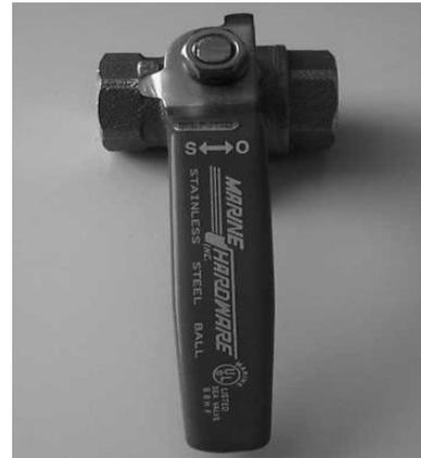
Ball valves (seacocks) are installed on the water intake for both the livewell and raw water system. The seacock must be in the open position for these systems to work. When open, the handle will be parallel to the valve. In the closed position the handle is perpendicular to the valve (see picture above). World Cat recommends that the seacocks remain in the closed position when not in use, or when the boat is left unattended to prevent the vessel from taking on water due to a plumbing failure.
