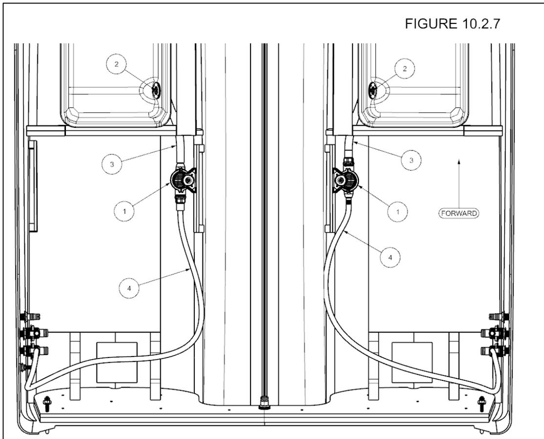
1) Diaphragm Pump 2) Fishbox Drain 3) Hose to Pump 4) Hose Overboard
