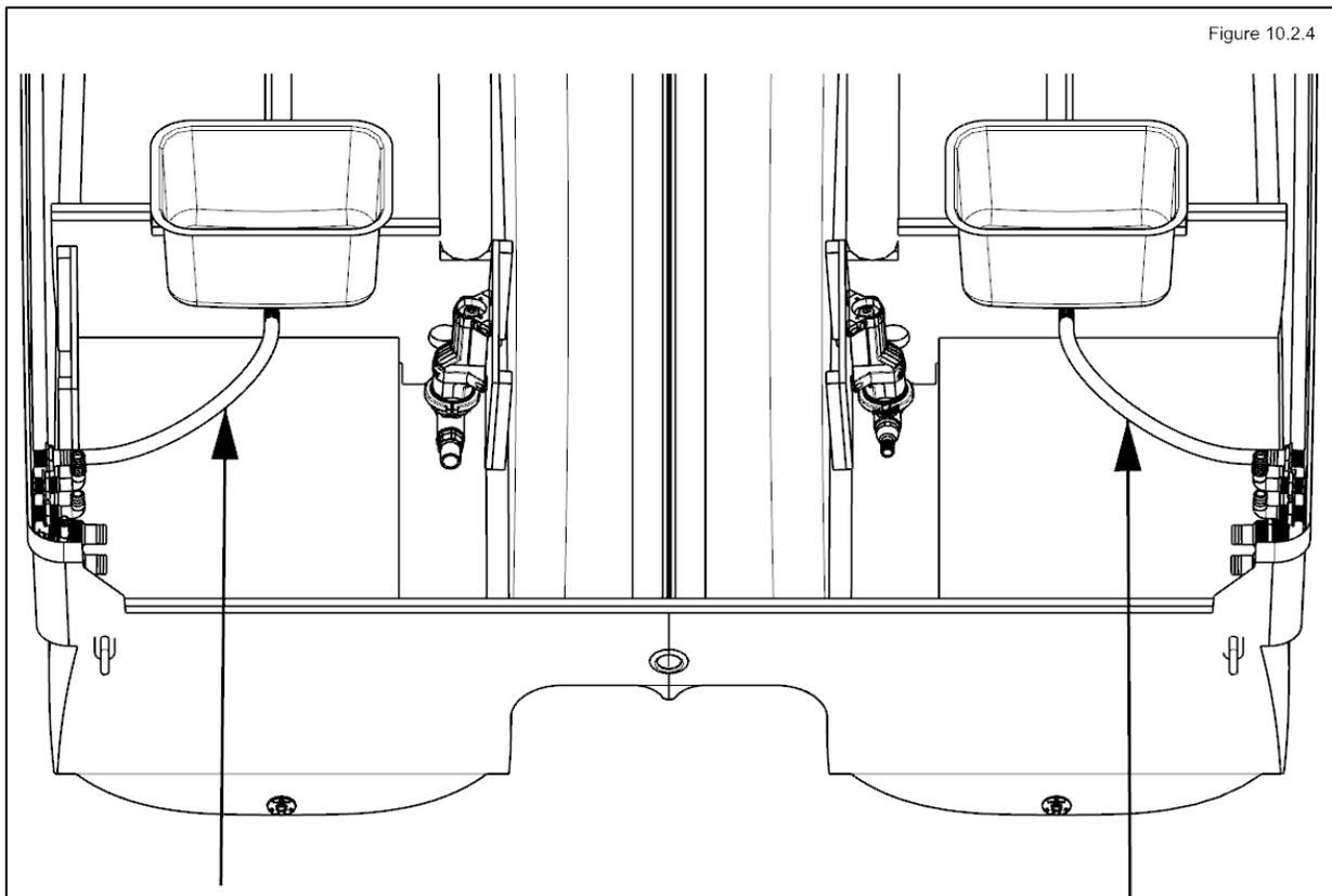
**Fishbox Drains** - The in-floor fishboxes on your World Cat are equipped with dedicated diaphragm pumps to efficiently pump liquids and small solids overboard. The pump and hoses are accessed through the mechanical room lids. (see Figure 10.2.5). The pumps are activated by a switch on the dash (see Figure 10.2.6). See Figure 10.2.7 for hose routing.
