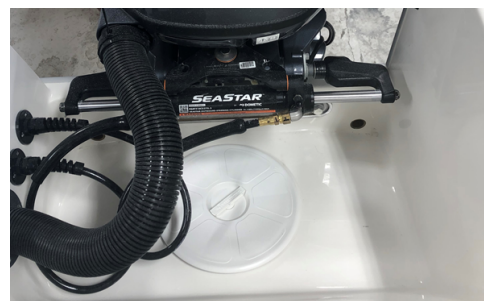
Optional steering system on 235CC, with power steering pump.
