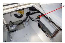
20 Ensure that the 200 amp House battery bank engine charging isolator circuit breakers in the aft bilges (mechanical rooms) are on for the engines to charge the House batteries while running.
