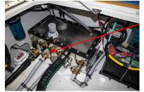
2 Open the raw water deck wash pump suction seacock on the sea chest.
