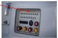
3 Ensure that the "House" battery switch is on at the main-D.C. panel to feed power to all of the manual circuit breakers on the D.C. panel except the "Continuous Power" circuit breakers which are fed direct from the house batteries all the time.
