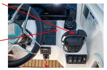
11 Once engaged, using the docking joystick will turn the engines in the direction necessary automatically to maneuver the boat as desired.
