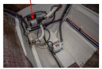
sewage holding tank is on the port forward guarter deck. The sewage tank vent is to the stbd. hull side.
