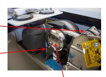
9 When safe insert the Lewmar wrench into the keyed hole in the face of the free fall cap and rotate clockwise to grip the gypsy and anticlockwise to free the gypsy
