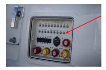
8 Ensure that the "Marine Head" circuit breaker on the main DC electric panel is on.
