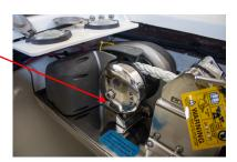
switch until the anchor is under free fall. If the clutch was left in a locked position the anchor will start to fall almost immediately. If unlocked it could take several seconds to fully re-engage the internal clutch. NOTE: Pressing the DOWN button for over 5 seconds will result in a longer clutch re-engagement time during the next UP command.
