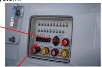
14 Ensure that the "Elect" (to feed the fuse block for the Yamaha CL7, NMEA 2000 bus. monitors, and other electronics) 50a, "COI 1" (to feed COI1 D.C. Loads) 100 a, "COI 2" (to feed COI2 D.C. loads) 100 a, "OI" (LROI 20a), and "C6" (5a Output Interface) manual circuit breakers are on at the main D.C. panel. These circuit breakers feed the D.C. loads and the Czone system.
