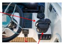
3 The trim assist function can be activated when the remote control levers are in the forward (F) position. The active indicator will be illuminated during operation. See page 36 of the Yamaha Helm Master Operations manual for information on setting engine speeds and the appropriate trim angle settings.
