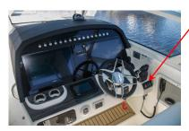
4 Operate the helm seat with the rocker switch to stbd. of the helm on the main control console.
