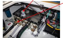
3 Ensure that the 12 volt "House" battery voltage is adequate (at least 12 volts).
