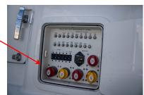
2 Check that the on generator 30 amp D.C. fuse is intact (on aft lower side of engine outboard).
