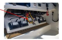
7 Ensure that the green network LEDs on the COIs are on indicating that the Czone NMEA network is intact.
