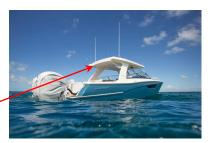
Do not operate the vessel with the Sure Shade extended. Operating the vessel with the Sure Shade extended could tear the shade and jam the mechanism so that the shade may not be able to be retracted. Do not leave the shade extended
