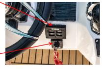
There is a multi-hub connector strip for each engine to interconnect all of the Helm Master components.
