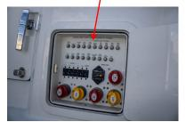
20 Ensure that the circuit breaker for the shore mounted receptacle box is off and turn off the main incoming 50 amp shore power circuit breaker by the inlet connection at the stern.
