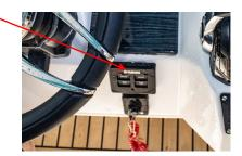
7 To lock the engines off place the EKS fob over the lock indicator, the beeper sounds once. This indicates the lock mode is selected and the ignition switch cannot be turned to "ON". When in lock mode, the EKS panel lock indicators blink. When the Ignition switch is OFF, or the Ignition switch is ON and the engines are not running, locking can be performed.
