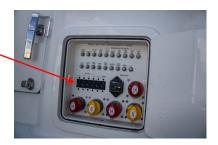
4 Ensure that the fuses in the fuse block under the console (fed by the "Elect" 50a circuit breaker on the main D.C. panel) are intact. The "Compass" fuse feeds the Yamaha/Garmin gateway interfaces (for autopilot, GPS); the compass light, and the head vent fan. The "Sonar" fuse feeds the fathometer function. The "AIS" fuse feeds the AIS system. The "VHF" fuse feeds the VHF radiotelephone. The "Monitor" fuses feed the
