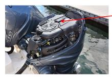
2 Ensure that the fuses in the fuse block on top of each engine under the cowling are intact.
