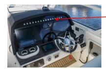
11 Turn on the "Raw Water" pump circuit breaker on the Czone touch screen or in the row on the top on the dash brow.
