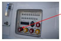
3 Ensure that the port start battery switch is on in the main D.C. panel
